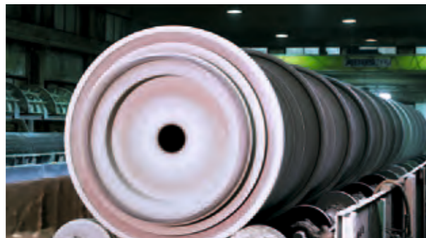
Compaction of the concrete in a rotational unit
