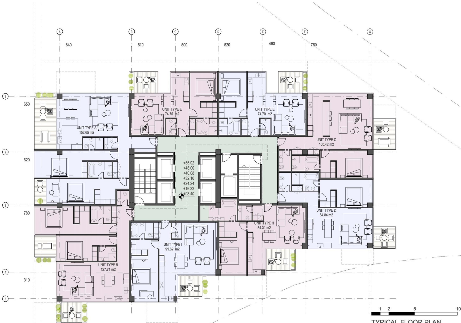
TYPICAL FLOOR PLAN TOTAL AREA | 931.34 TOTAL COMMON AREA | 137.96 M2 NUMBER OF BLOCKS | 8
