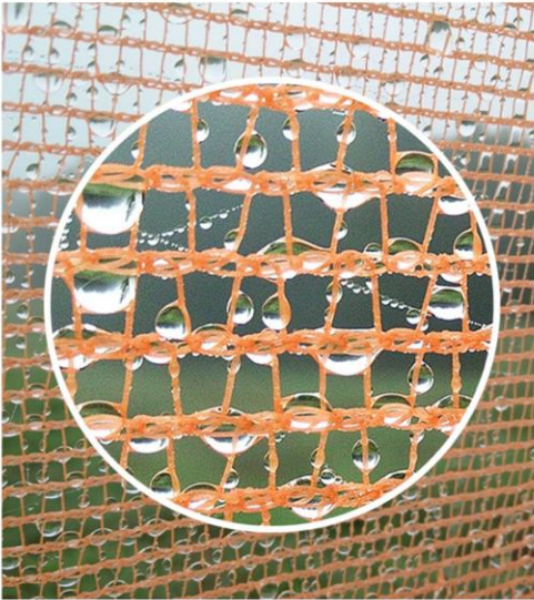
Dew Towers Fog Nets | HDPE Mesh
